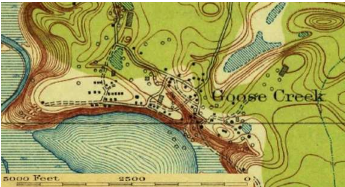
Image 2. The same 1916 map enlarged to show features in the oil field. There are fifty round circles which represent oil wells and the black squares represent structures. The shaded rectangles are earthen oil pits. Judging from the number of oil wells, the survey was probably done in
